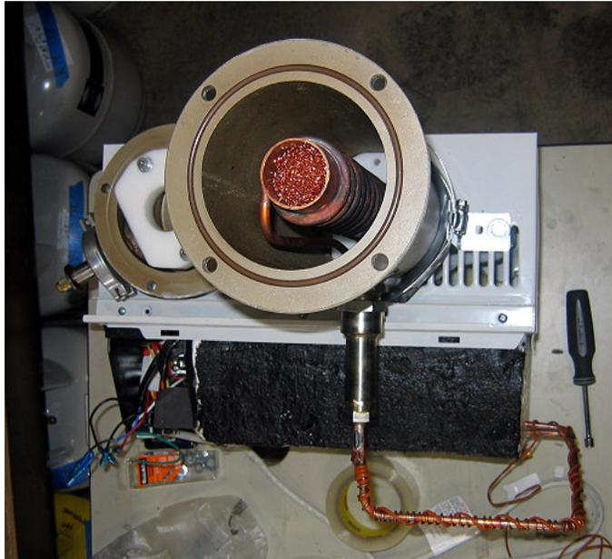
Here's a birds-eye view of the connected cold trap (modified vacuum pump exhaust filter housing). Inside can be seen the evaporator assembly which consists of a 12" length of 1 5/8"od copper tubing with 1/4"od tubing coiled around and brazed to its outside surface.
