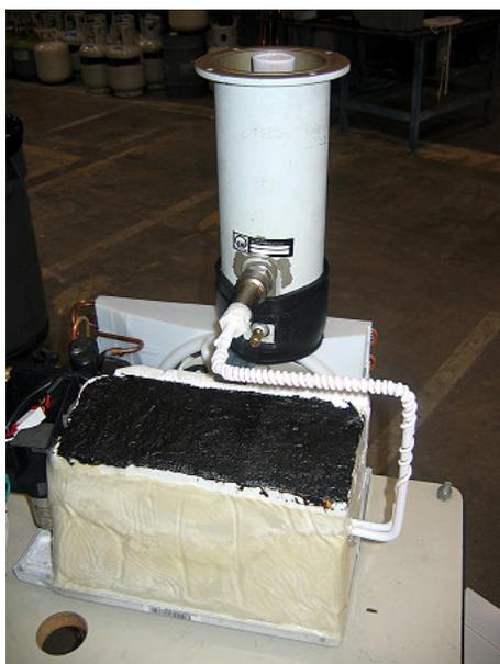
Next the cold trap was connected, leak checked, evacuated, and the refrigerant charge was added (placed the unit on an electronic charging scale).
