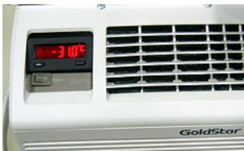
This temperature (-31°C) is well beyond the -9.0°C requirement for condensing alcohol at 10 mmHg (lowest possible pressure level with a standard mechanical vacuum pump). Success!
